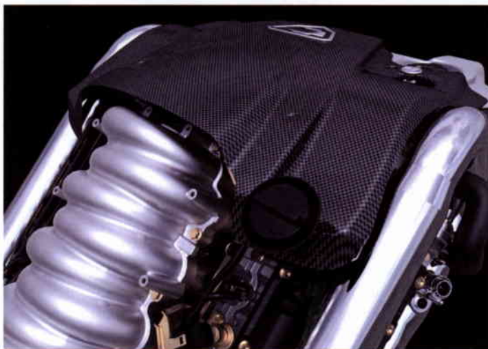
Engine detail shows swirling air/petrol induction chamber and electric engine management unit.
