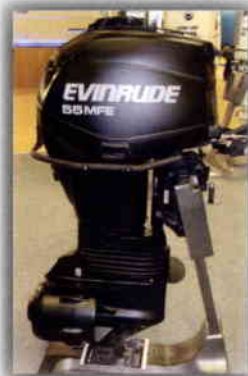
Evinrude's multi fuel, jet drive outboard – the 55MFE
